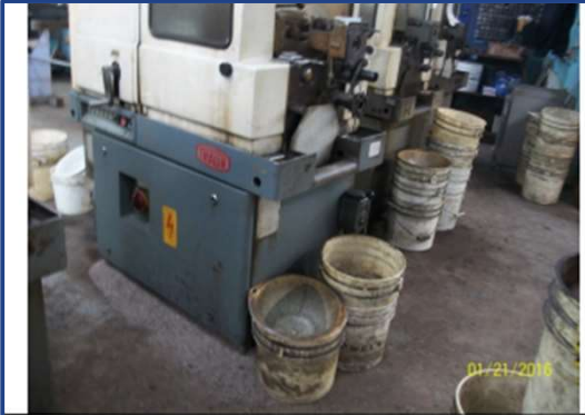
Photograph 2: Absorbent at base of one of the machines.
