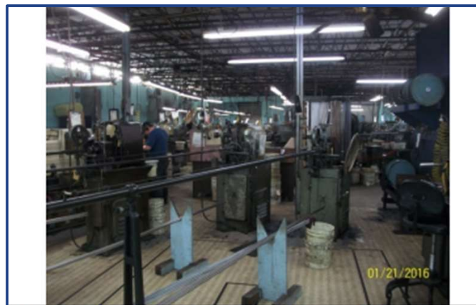
Photograph 1: Open shop area with many Swiss screw machines.
