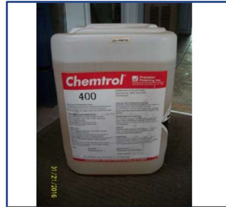
Photograph 8: Finishing compound used in tumbler: pH of concentrate is 1.0 – 2.0 according to MSDS.
