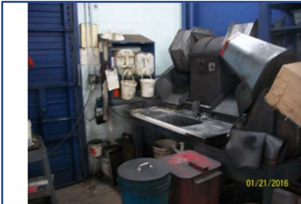
Photograph 4: Sink, tumblers and dip washers.
