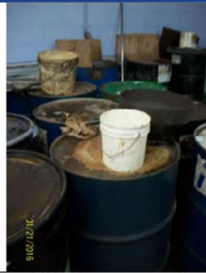
Photograph 10: Empty drums and waste drums in adjacent building a. Note open funnel behind white pail on one of two waste drums.
